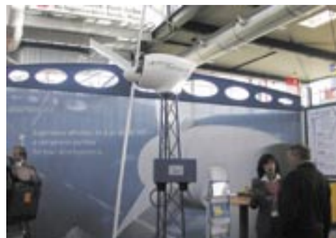
Prototype of a 5 kW wind power turbine for the coupling to the public grid and for the use in small autonomous supply grids
