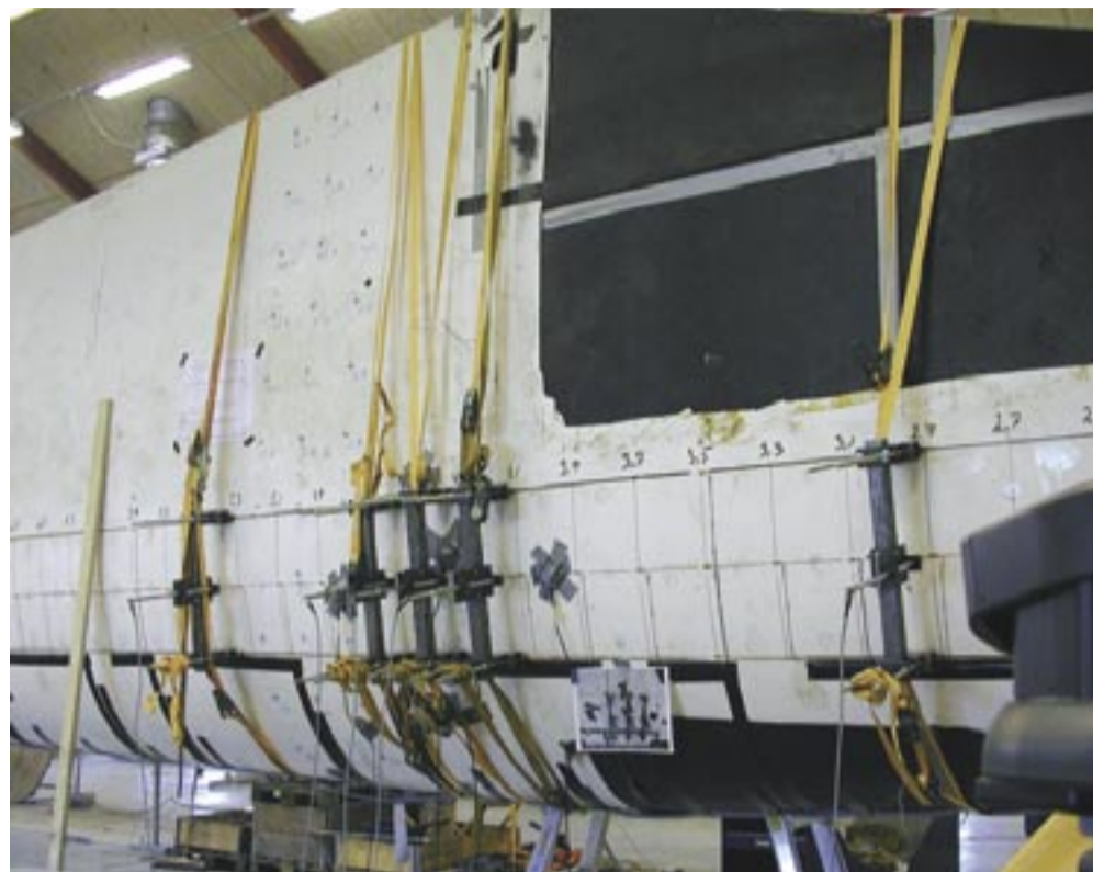
Buckle sensors on a wind turbine blade during test
