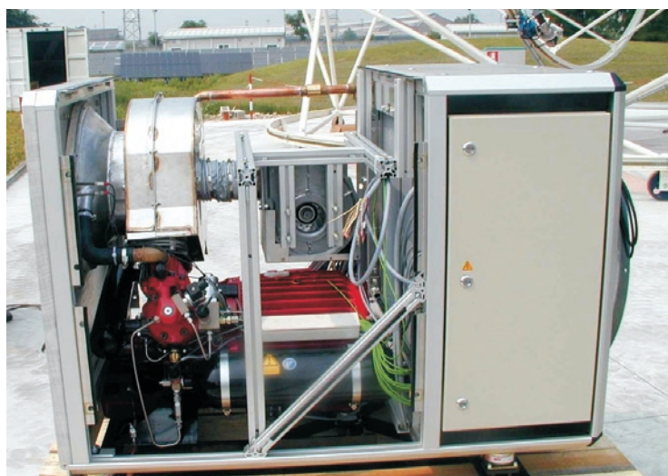
The SOLO 161 Stirling motor solar unit open before the installation
